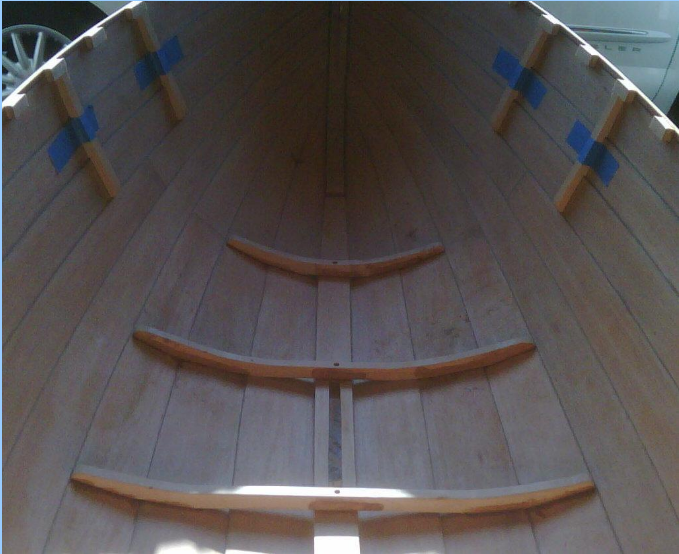
Alder half frames are installed in the bow. Alder spacers are ready for the Mahogany inwale to be installed.
