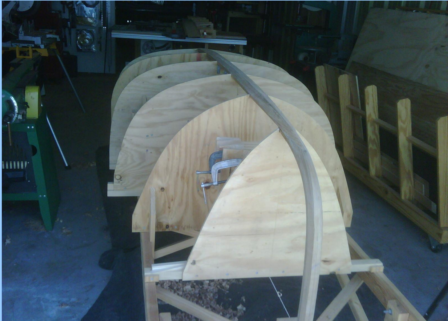
First Celebration: Stem and transom are laid up. (White Oak stem and Western Red Cedar keelson are laid up on the plywood molds.)
