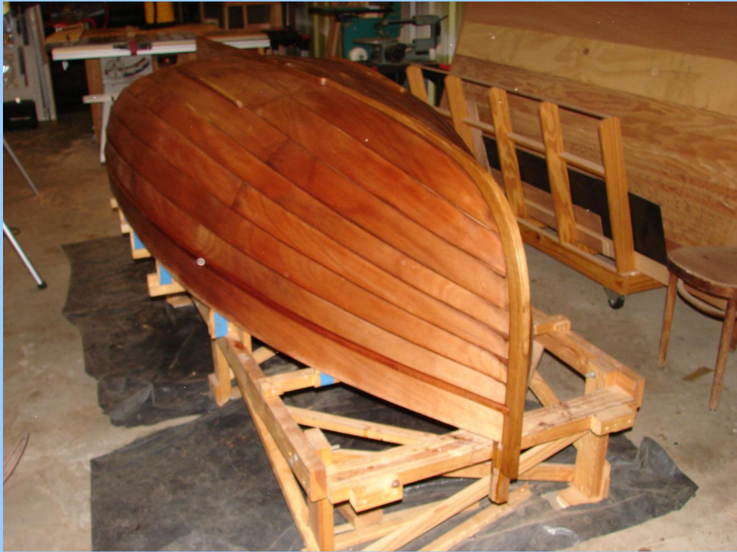
The sealed hull showing White Oak stem, Okoume plywood strakes and Mahogany rub rail.
