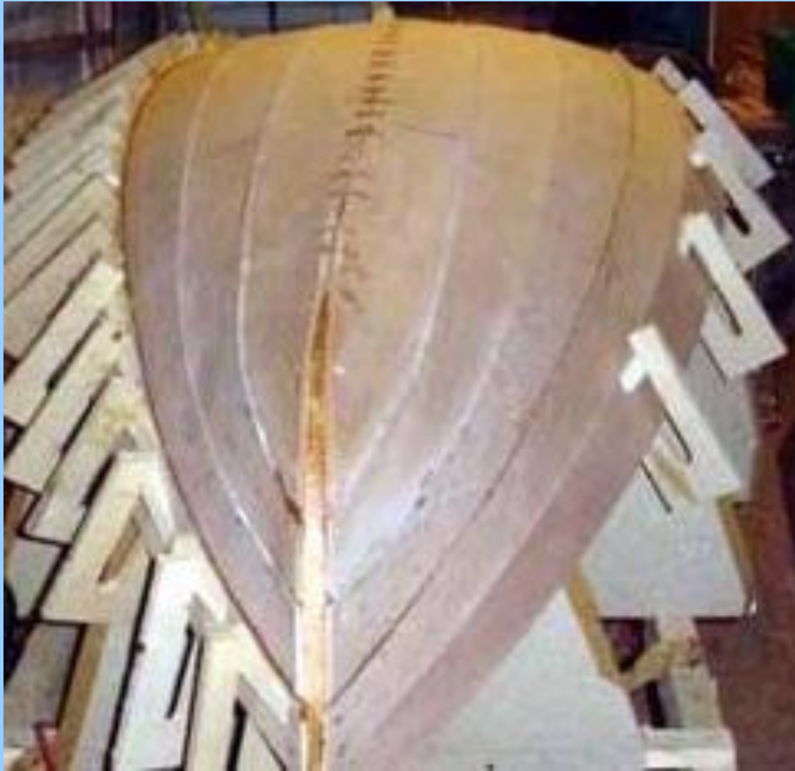
Strakes installed using shop-built C-clamps and wedges
