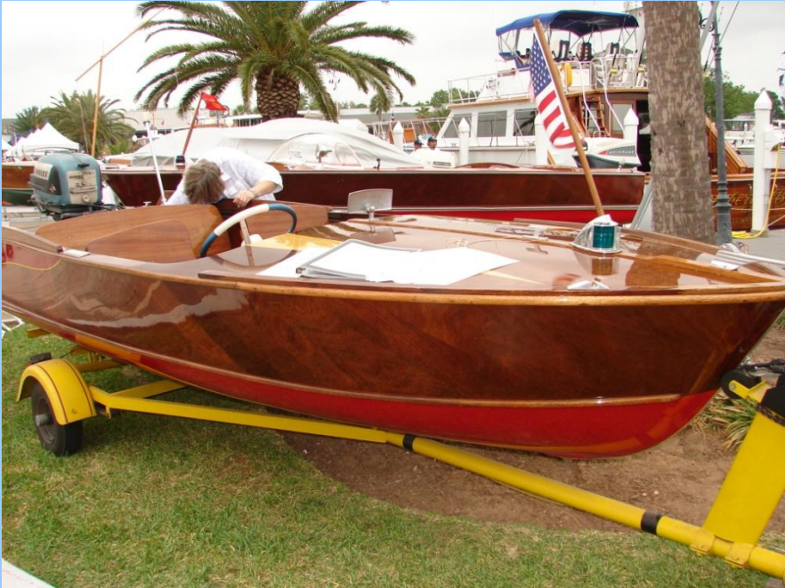
Hot Molded “Yellow Jacket” runabout built in Denison, Texas using monocoque airplane construction methods
