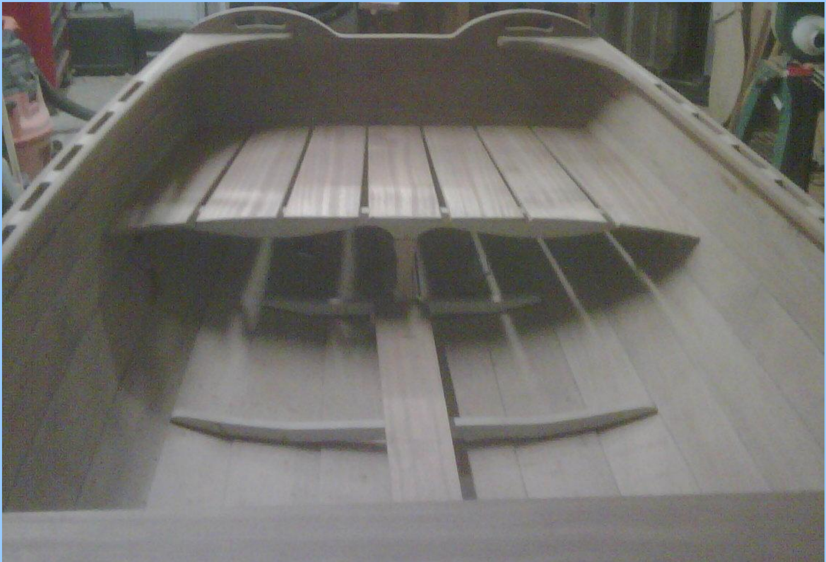
Mahogany inwale is installed. Mahogany stern sheets and center thwart are laid up for final fit.
