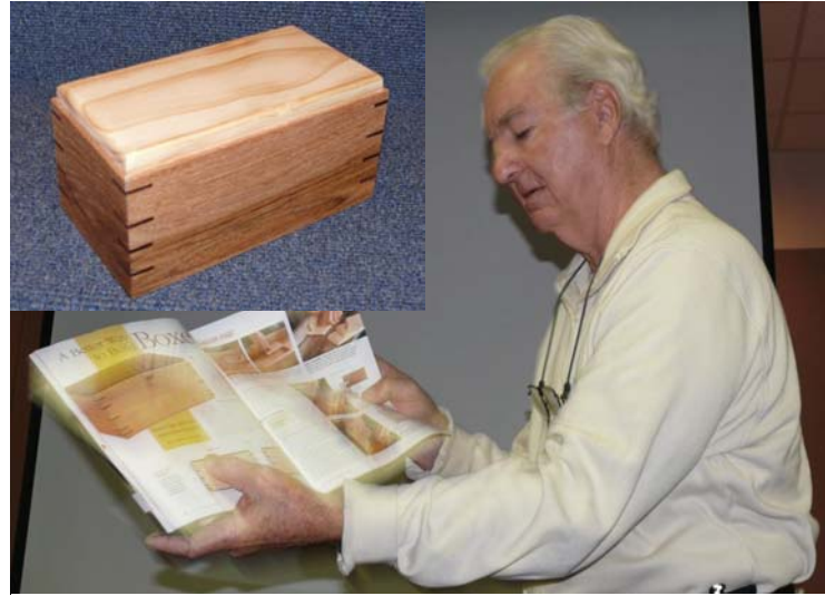
Ridg Gilmer read the article "Better Way to Build a Box" from Fine Woodworking Magazine, and decided he could do that! Ridg's box is oak with a birch top & walnut splines.
