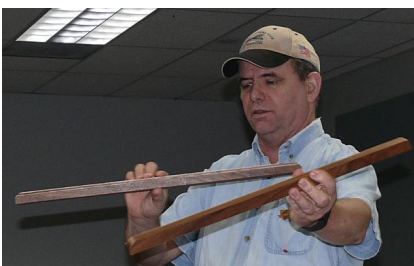
Mark Bolinger showed Club members plane sticks which you can use to verify the flatness of a surface that you have just planed.
