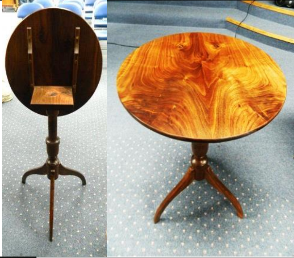
Josh Nichols designed this tilt table this walnut table which features flying dovetails to hold the legs securely. The walnut grain makes a beautiful table top.
