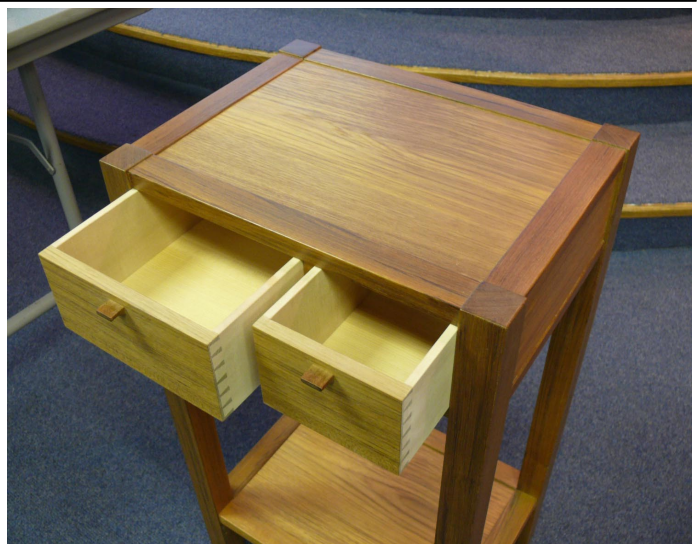
Clark Kellogg made this end table as an experiment and a prototype before a larger piece he had to make. Using predominantly Teak and other wood for contrast in color, drawers of two different sizes for better utility and slip tenons and lpe handles, Clark crafted a simple yet unique end table.
