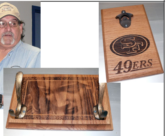
David Garcia held up some laser engraved plaques that he crafted of solid oak. A hidden magnet catches bottle caps, of course after the bottle has been opened. David finished with two coats of oak stain, no poly, just stain.
