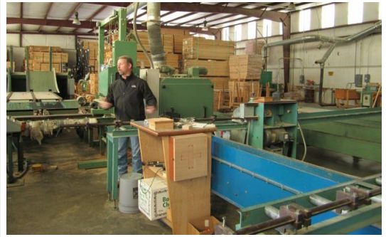
Wood enters the plant at the gang rip saw and cross cut saws.
