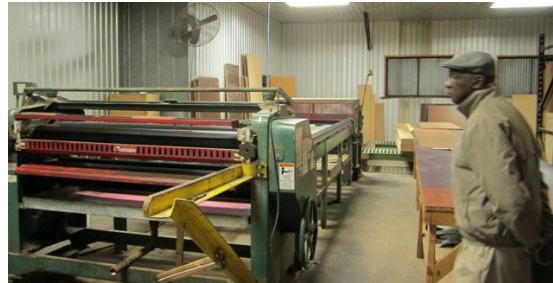
Laminates are applied to the sheet goods.
