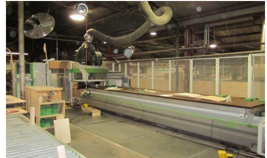
One of several CNC routers.
