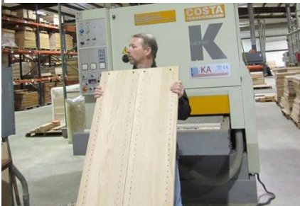
A thickness sander (behind) near the end of the line.
