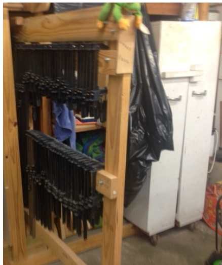
Larry found a way to make full use of the slightly elevated walkway that most garages have by building pullout storage cabinets and racks for things like clamps.
