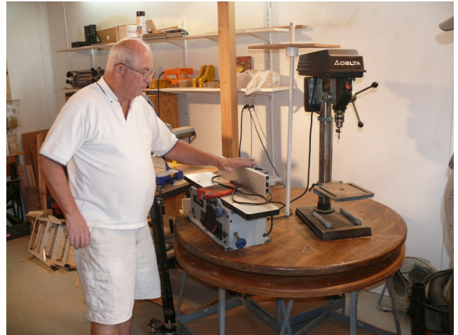
Larry explains that using a large lazy Susan for table top tools works great in a small shop space.
