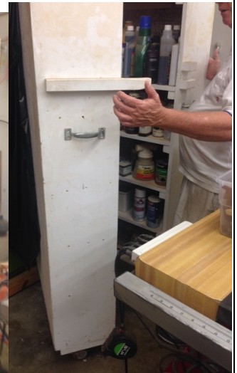
Larry found a way to make full use of the slightly elevated walkway that most garages have by building pullout storage cabinets and racks for things like clamps.
