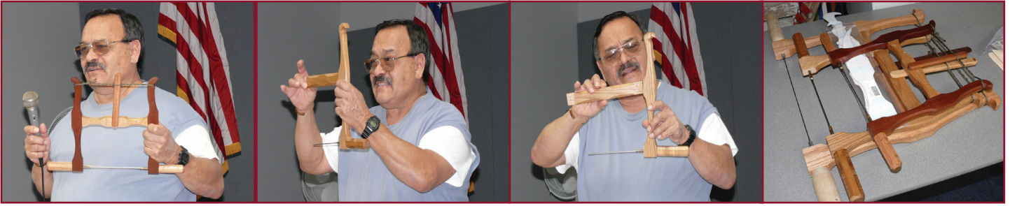
Fred Sandoval, a longtime member of Woodworkers Club of Houston, provided oodles of tips for making bow saws. Ash and White Oak are good wood choices but maple is not. Fred recommends quarter sawn wood. All the joints are mortise and tenon but are not glued. The tips of the tenons are rounded to allow joint flexibility.
