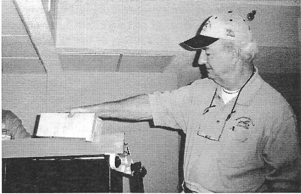
Ridg Gilmer showed his adjustable "short fence" for use on his Delta Unisaw. It's used for narrow pieces.
