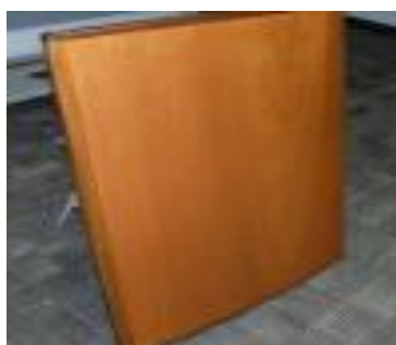
Michiel Tijsseling - Boat hatch from teak, and okoume and finished with Cetol Marine
