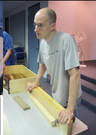
Mark Sweigart created this Moxon Vise in maple. He incorporated wheels to raise and lower the vise.
