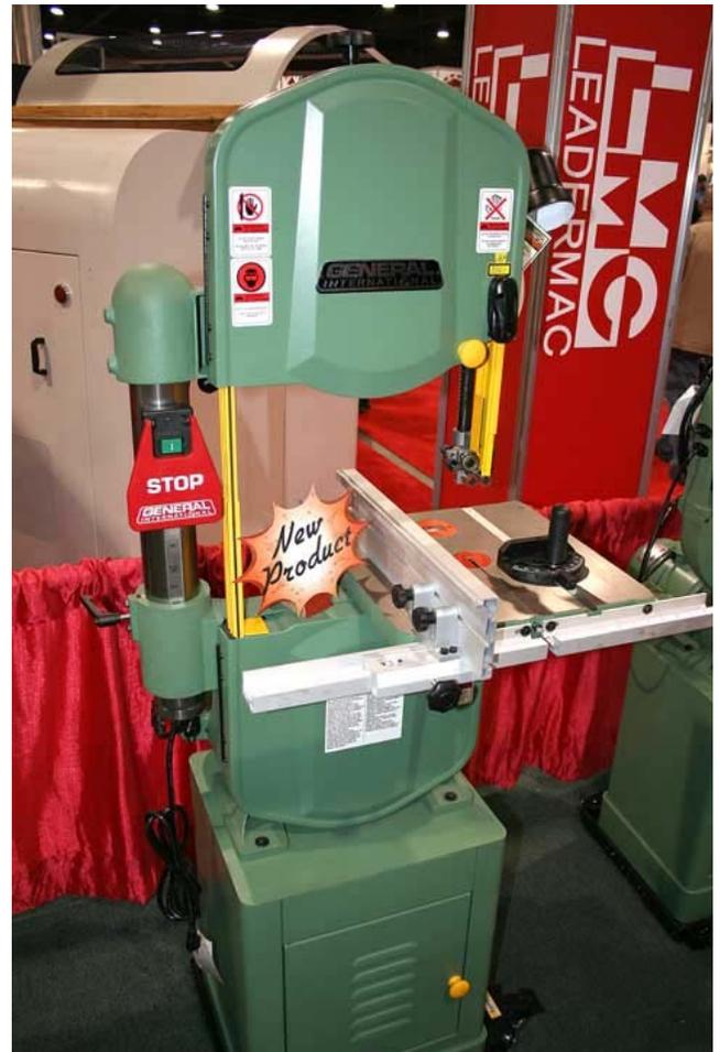
At first glance, it looks like a drill press and a typical 14” bandsaw were involved in a bad accident, or somebody at General was fooling around with a welding torch and way too much time on their hands. But actually, it’s a pretty good idea. This new saw, which will list around \$1400, allows you to make regular cuts with a 93” blade, or crank up the head to increase your ability to resaw with the 102” blade. Cool!
