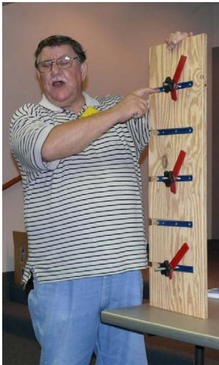
Feeling “ripped off” by that crooked piece of lumber you bought at the hardware store? Andy Andersons clever jig allows you to rip a straight line on a board. T-tracks secure the hold-downs. Now that’s the straight truth!
