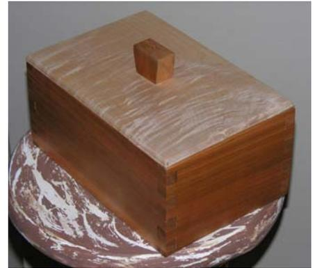
Also, I'd use two routers next time, one for pins and one for tails. In my project I cut all the pins first, then the tails, but changing bits and bit heights back and forth was a hassle.
