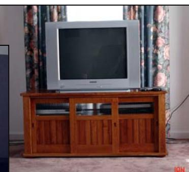
**Mark Bolinger** brought in one of the panels that would ultimately be one of the sliding doors to his entertainment stand. He included windows so he could use slats that were already cut from a previous project. Mark explained how the bottom is a thin rail and the top is beveled to allow easy removal of the door. The stand is finished with Danish oil and polyurethane. Looks great, Mark!
