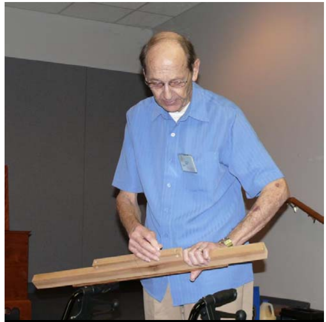
It's all fun 'n games to Marcus Brun when he uses this jig to align holes for the games he creates.
