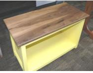
Following an existing plan rather than creating a design using SketchUp, Mark Womack made this bench for his niece to place under her window. Mark used poplar and plywood with a walnut top and then assembled with pocket screws. Mark used a mallet to drive 3/8 dowels into the pocket hole spaces then used a flush-cut saw to cut away excess.
