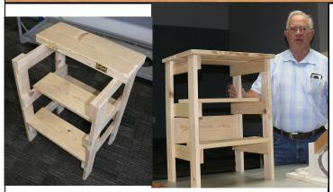
Stepping up to the task, **Chuck Graham** made this combination table/step stool of pine. The design came from an old woodworking magazine. The top hinges allow him to change between stool and step stool. It will be for his garage so he didn't finish it.
