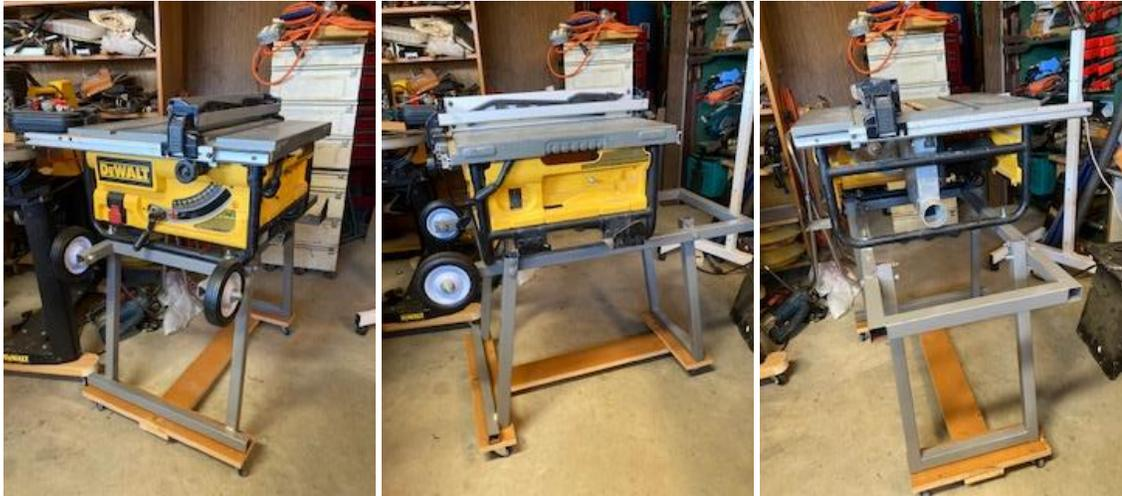
It is a mobile base for a 10" Dewalt table saw. The base is designed to fold up the legs and then roll the saw to transport it or use it at the jobsite. The base is made of 1 1/4" steel square tubing, 1/16" wall. The length of the base frame is 36" and has a width of 16". The legs are designed to fold up underneath in order to transport. Once you
