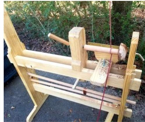
The spring Pole lathe is a Roy Underhill design. Always making sure the designs stand the test of time, the construction is made of yellow pine, with the springs are made of hickory. The dead centers are made of O1 drill rod steel. — **Pamela Gideon**
