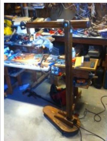
This is an adjustable boom shop light I made a few years ago. The reason I am showing again is that I put casters on it and it is much easier to move around when I need additional light in an area. Easy to make, light is from an old tract lighting system that I recycled.—**Mike Turner**
