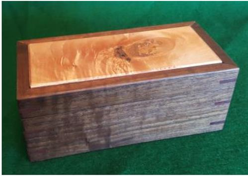
**Andy Tofuri** — With a bit of left-over walnut, I decided to make a box to keep in practice. I found an old scrap of curly maple with a knot in it that I had cut out of a board. Stabilized the knot with some CA glue. Made a wood hinge from 1/4" dowel & 1/16" brass rod, but didn't get the groove just right so I had to carve out a bit on the back for
