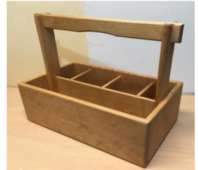
**Chuck Meeder**—These two tool totes were made from cutoffs from old projects. One is red oak, the other maple; both finished with teak oil. They are 15 inches long. The handle on the oak one is wrapped in braided nylon cord with additional finish applied over it.
