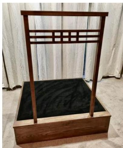
A new conductor's podium for the University of California - Irvine (actually ships out today - 6/4). The box is 42"x42"x10", and top of the railing is 42" above the platform. It is ash stained with walnut gel stain and a poly top coat. The platform is commercial carpet over an anti fatigue matting on 3/4" plywood. The railing system comes out, and there is an insert for when it is not used.—**Mike Hardy**
