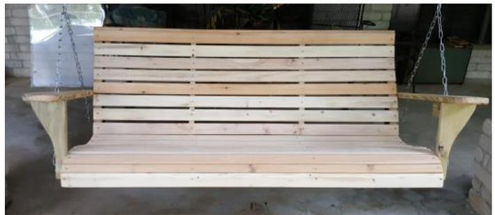
Out of scrap bodark Sam Grice turned some cups. Also, Sam ran some cedar and treated pine board pickets through a planer, ripped to width and made a porch swing. Because of the moisture in the wood Sam disabled his Sawstop sensor – yup – the light was blinking – he didn't want a \$50 swing to turn into a \$250 swing.
