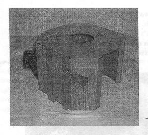
Left: This dust collector was built by Hunter Malson. Hunter built it out of 1/4 plywood and used only glue and a Porter Cable pin nailer in its construction.
