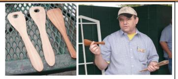
From the hand tool splinter group, **Mark Bolinger** crafted some soup spoons – you know – for the lumps. Mark explained how he first roughed out the spoons by band saw then used a scraper followed by a spoke shave for the finer work.
