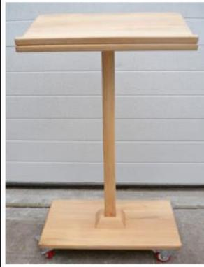
Birthday present for my wife: a dictionary stand on wheels. Sycamore, with one coat of tung oil to show the grain more, dried for 3 days, then finished with water based urethane. I just didn't like the effect I got with an assortment of stains I tried. Any suggestions? Mortise and tenon joints to attach the post. — **David Janowitz**
