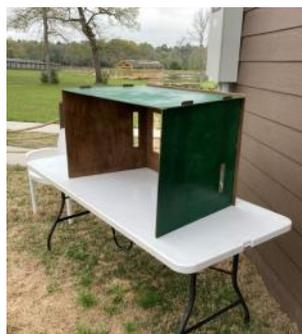
This is a project I put together to help my wife during scout tours at the Wolf Sanctuary we volunteer at. It is made out of Luan and is cut with inter-locking tabs for ease of putting together and breaking down. Tabs on the back slide and lock, the tabs on the top are more of a locator.
