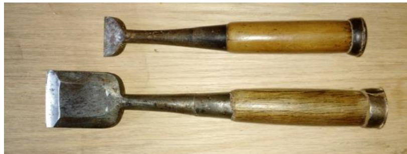
At the top is what used to be an excellent chisel, but is now just, to be polite, a nub; the lower one is a still usable example for comparison. Why was this chisel still in the tool roll? It's too short to sharpen. It's too short for self-defense. In a stretch, one might use it as a scraper but there were six of them. Conclusion: the old carpenter couldn't bear to throw it out. Worse: why do I still have the nub? Conclusion #2: I need a twelve step program for tool addicts.
