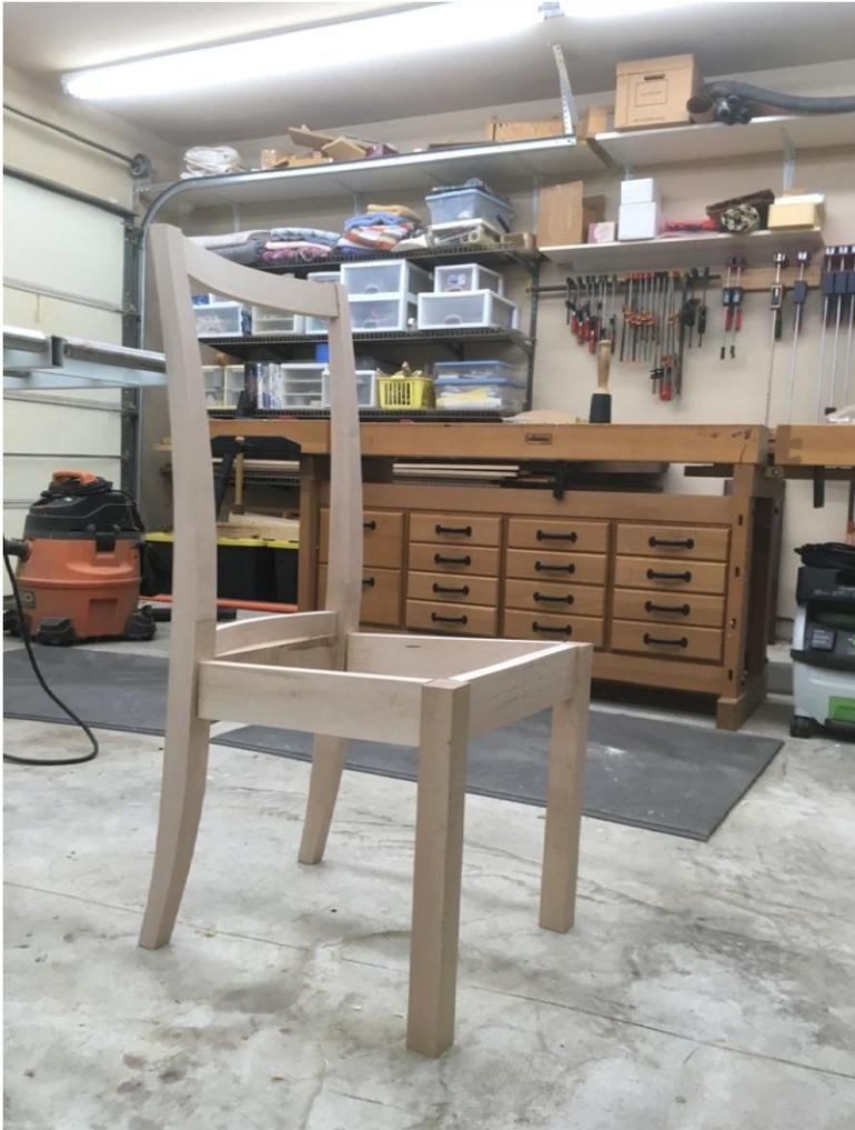
Here is what it looked like with the back legs shaped and the top and bottom rails of the back fitted in position
