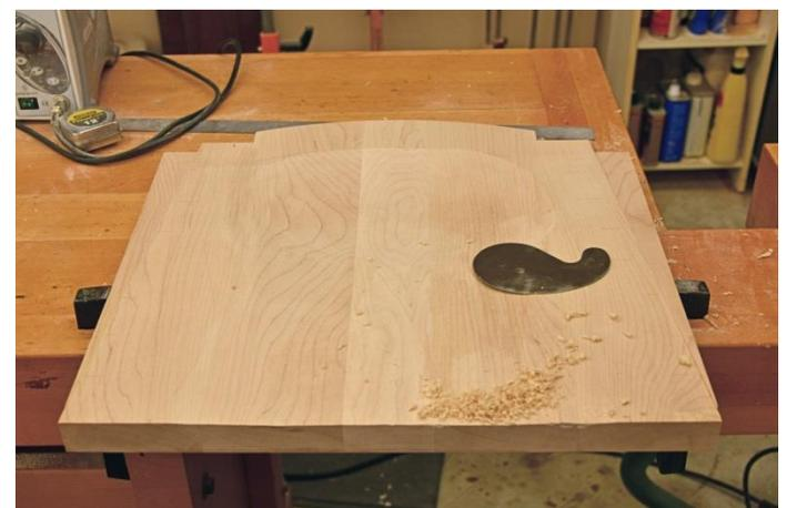
Then smooth the contours with a rotary carver and a spherical burr, followed by random orbit sander until carving marks are gone, then final scraping to even out a few bumps
