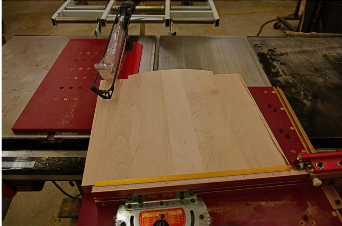
Cutting the angled sides to the seats was straightforward using the table saw and Incra miter gauge
