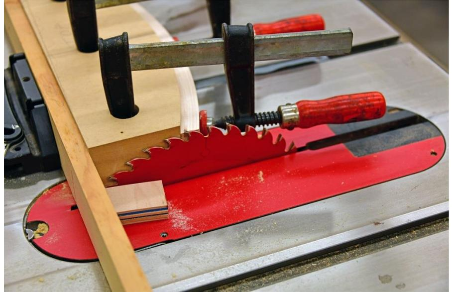
The rail was clamped to the jig, one end of the jig set against the stop block, and the first end trimmed.
