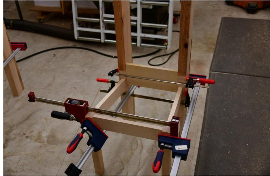
With the chair still clamped up, the exact size of the back rail can be measured.
