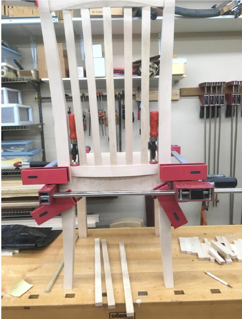
Back slats have 3 different lengths and most have compound angles at both ends
